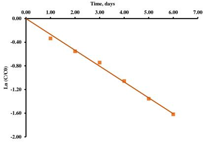
Fig.7.First order kinetic model for color removal in a textile industry effluent for the optimum nutrient dosage (50 g), dilution ratio (10), pH (7) and contact time (6 days)
