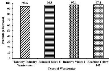
Fig.6. The percentage reduction of color in a textile industry wastewater and in an aqueous solutions using *Lemna minuta L*. against optimum nutrient dosage (50 g), dilution ratio (10), pH (7) and contact time (6 days)
