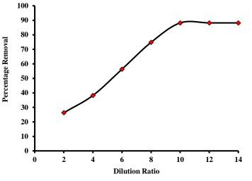
Fig.4. The percentage reduction of color in a textile industry wastewater using *Lemna minuta L*. against dilution ratio
