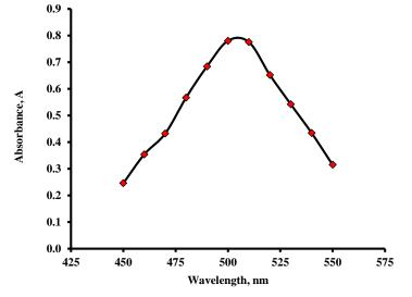
Fig.1. Absorbance curve for textile industry wastewater
