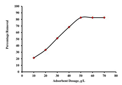
Fig.3. The percentage reduction of color in a textile industry wastewater using *Lemna minuta L*. against nutrient dosage
